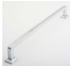
Bronte Handle Polished Chrome Item No: B[96/128/256]PC Length: 115/147/275mm Centres: 96/128/256mm Projection: 34mm
